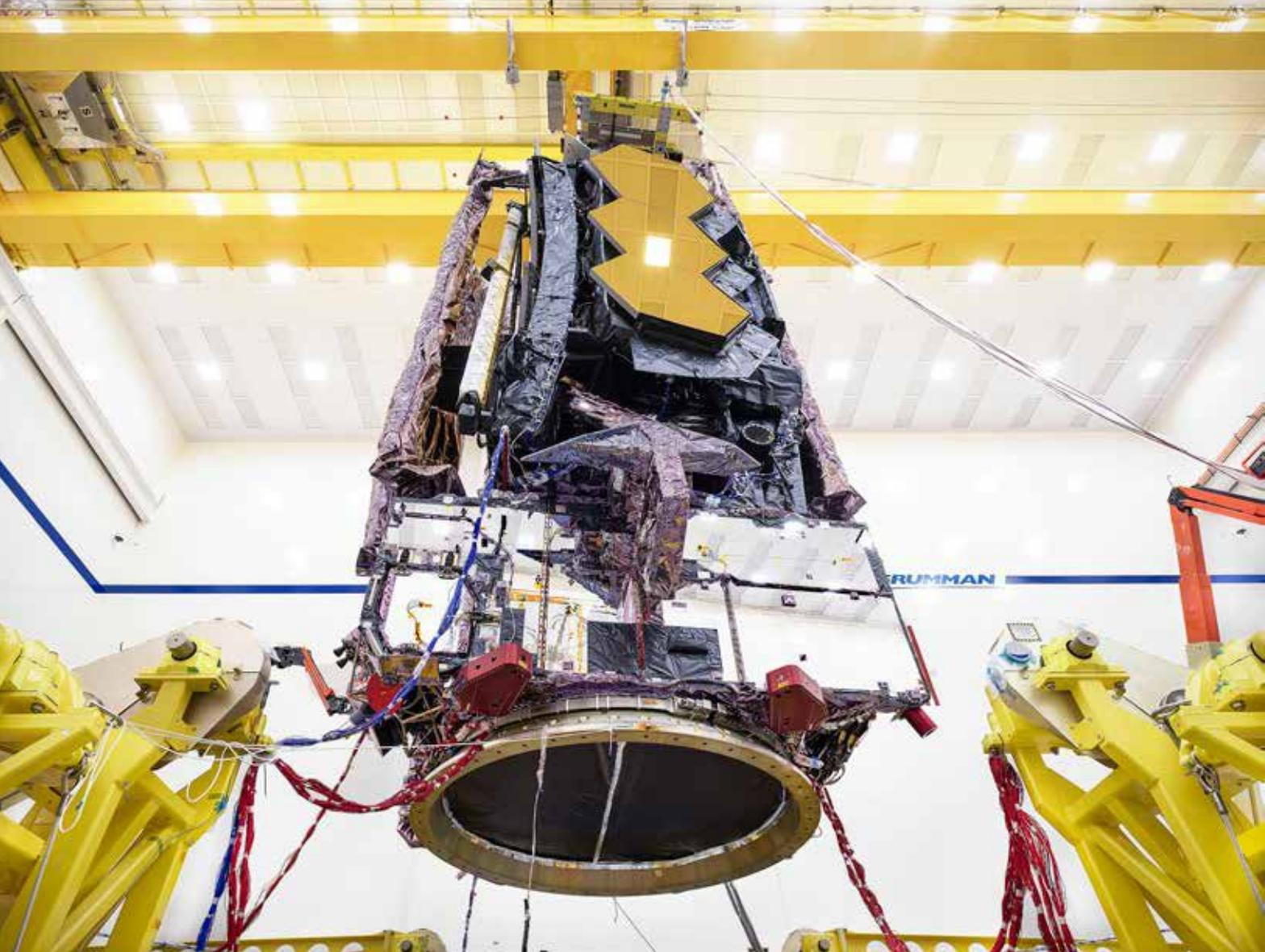
▲ **JWST in its launch configuration** at the Northrop Grumman clean room in California, where engineers in October completed the acoustic and vibration testing that replicated the forces the observatory will experience during launch. Plans call for enclosing the observatory in a protective container early next year and shipping it on a barge to French Guiana for fitting inside the payload fairing of an Ariane 5 rocket.
